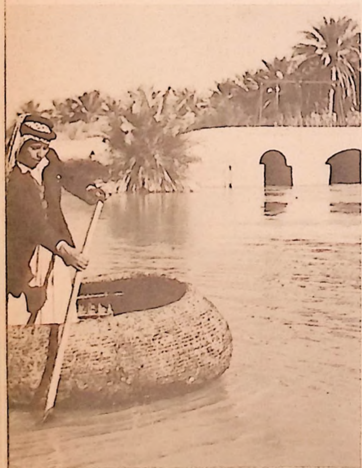
The centuries-old "gufa," bamboo fibres held together with pitch, is still seen on the Tigris, another reminder of the Land Between the Rivers which has given Iraqis a cultural and historical unity.
