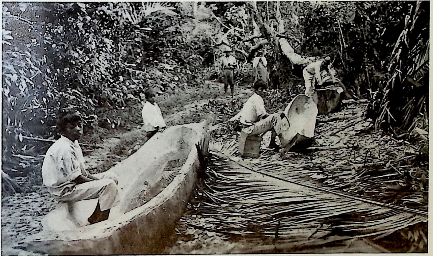
Dories are made from a solid log and the work of chopping out the inside is done right in the jungle of British Honduras.
